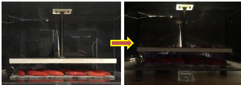
Gambar 2. Proses Pemberian Perlakuan Cold Plasma
