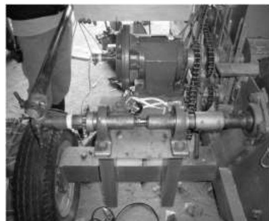
Gambar 1. Pengukuran kalibrasi strain - torsi
